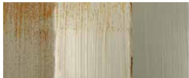
Typical brush application of traditional epoxy mastic coatings (left & centre) and Jotamastic Smart Pack (right) after continuous exposure in a salt water chamber.
