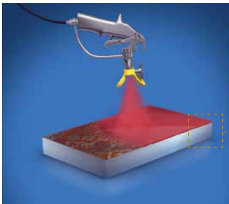
1. Jotamastic is applied to an aged coating in sound condition prepared to minimum St 2 (or even moist). Waterjetting prepared surfaces with early flash rust are acceptable.
