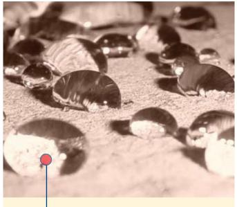
Water drops not absorbed by the concrete substrate indicate lack of preparation or contamination.
